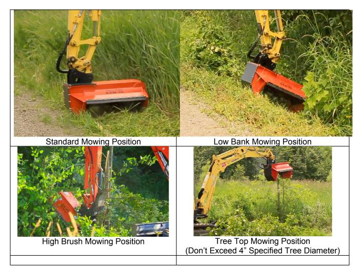
When operating EX Mowers on an excavator, care should be taken to never rotate the mower back towards the operator when the blades are spinning.
